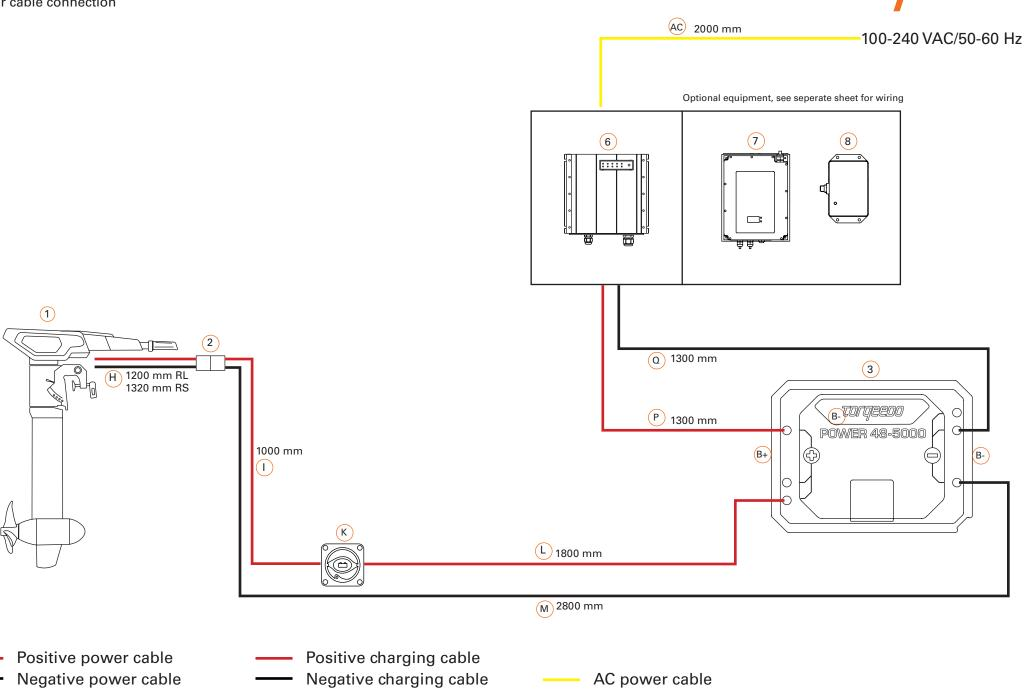
Installation Drawing: I39 Version 1.2 System ground connection
