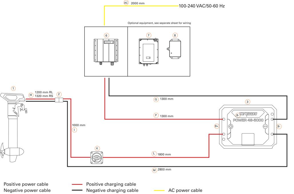
Installation Drawing: 108 Version 1.1 System ground connection
